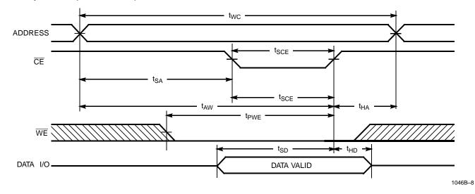
Write Cycle No. 2 (WE Controlled, OE HIGH During Write)<sup>[14, 15]</sup>
